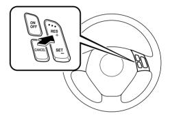
Your vehicle has a tap-up feature that allows you to increase your current speed in increments of 1.6 km/h (1 mph) by a momentary tap of the RES/+ switch. Multiple taps will increase your vehicle speed 1.6 km/h (1 mph) for each tap.
